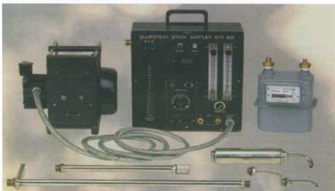
FIGURE-3 STACK EMISSION MONITORING KIT
